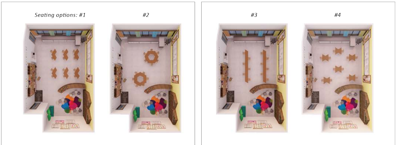
Layout options for configuring the classroom space for closeness and social distancing
